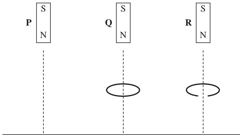
Three identical magnets **P**, **Q** and **R** are released simultaneously from rest and fall to the ground from the same height. **P** falls directly to the ground, **Q** falls through the centre of a thick conducting ring and **R** falls through a ring which is identical except for a gap cut into it. Which one of the statements below correctly describe the sequence in which the magnets reach the ground?
